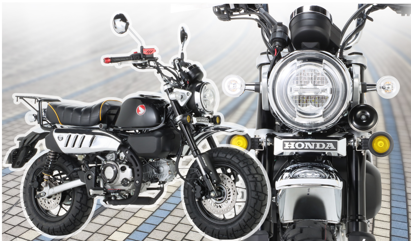
Emblem added, and horn relocated to left side of headlight.
